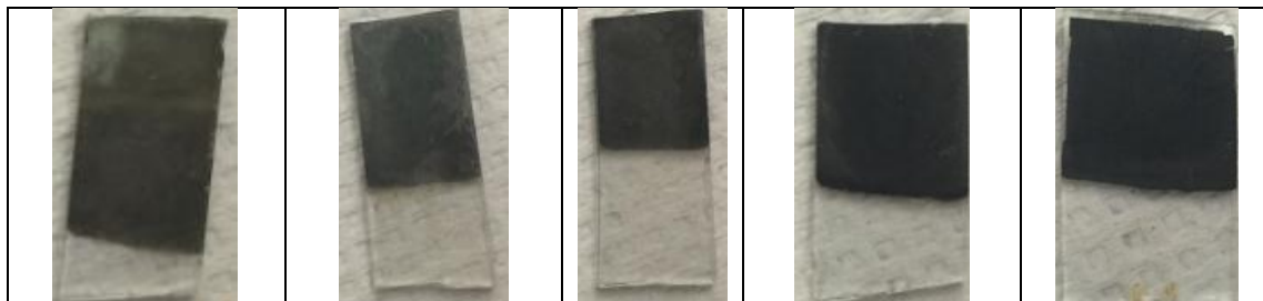
Figure 15. Photographs of MoS 2 -PPY composite films deposited at 8 mA/cm 2 current density as a function of time (30 sec, 1 min, 2 min, 5 min and 10 min).
